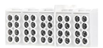
Power distribution block 5-p screw clamp Number of poles 5, Nominal current 80A, Connection type Screwing, Mounting method DIN rail, Number of connections total 20, Number of connections < 6 mm² 0, Number of connections 10 mm² 0, Number of connections 16 mm² 0, Number of connections 25 mm² 20, Number of connections > 25 mm² 0, Contact safe, Height 65,9mm, Width 102,4mm, Depth 45,5mm
