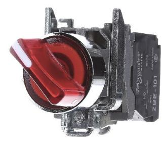
Illuminated selector switch, 2 positions, 1 NO contact + 1 NC contact - Thumb-grip switch 1NO/1NC...
