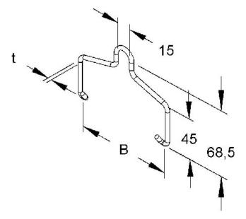
Suspension bracket - Ceiling bracket for cable tray REBA
