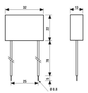
Capacitor module for up to 15 illuminated pushbuttons - Capacitor 1µF 026.00
