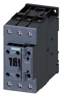
Contactor 22kW/400V, 1NO+1NC - Magnet contactor 51A 110VAC 3RT2036-1AF00-1AA0
