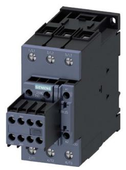
Contactor 22kW/400V, 1NO+1NC - Magnet contactor 51A 110VAC 3RT2036-1AK64
