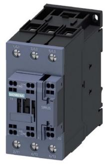
Contactor 22kW/400V, 1NO+1NC - Magnet contactor 51A 83...155VAC 3RT2036-3NF30
