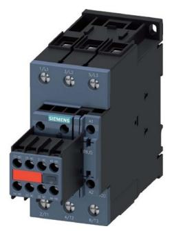
Contactor 30kW/400V, 2NO+2NC - Magnet contactor 65A 230VAC 3RT2037-1AP04-3MA0
