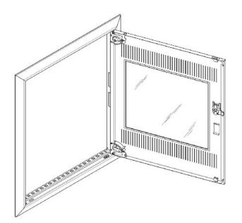
Blind frame with media door for UP-VT, 2x4 rows - Door for cabinet 550mmx650mm steel GBRU24TM
