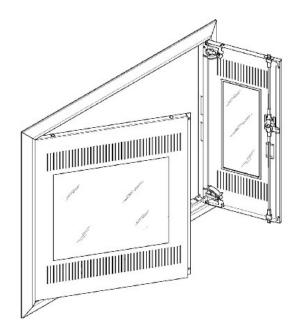
Blind frame with media door for UP-VT, 3x4 rows - Door for cabinet 800mmx650mm steel GBRU34TM
