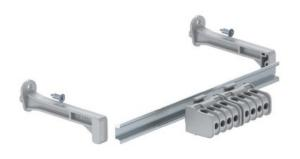
Terminal strip set with screw terminals KL-X16 06-16 rated current In 100A, rated voltage 450V, number of poles 5, number of terminal points per pole 4, other color, terminal strip set for the small distributors of the SDB series. The sets can be used to extend and equip empty small distributors of the SDB series
