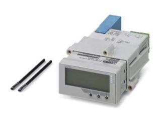
Digital display FA MCR-EX-D-2907216 Degree of protection (IP), front IP65, operating temperature -20 ... 60°C, front width 96mm, front height 48mm, installation depth 175mm, multifunctional Ex-i process indicator in switch panel installation housing for monitoring and display of analogue measured values. Universal inputs allow connection of current, voltage, RTDs and TCs. Two relay changeover outputs and one analogue output.
