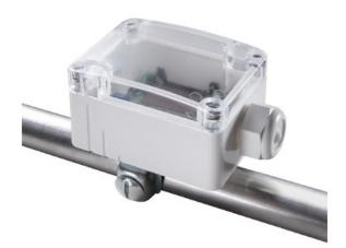
Battery-and wireless contact sensor for temperature control in connection with the receiving interfaces SRC-x and higher-graded control systems. For measuring temperature on pipes and arched surfaces. Detection of measuring values via the higher-graded control systems. Transmission to receiver by means of radio telegrams according to enocean standard. With integrated temperature sensor and solar energy storage for maintenancefree operation.
