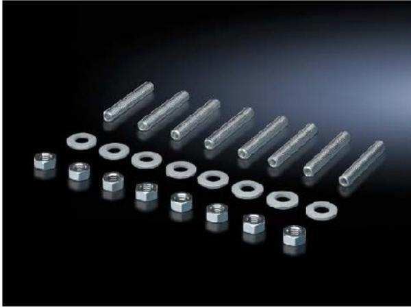
SV bolt VB set for Maxi-PLS 3200 SV 9676.981 (PU8) Material steel, other material quality, surface electrogalvanised/electrolytically galvanized, thread type PG, thread size (metric) 12, thread pitch 1.41mm, full thread, length 40mm, connection bolt M12x40 for connection sets /Connection angle (Maxi-PLS3200), including spring washers
