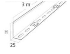
Divider COT 50 GS, divider height = 50 mm, length = 3000 mm, version = L-profile, fastening perforation = yes, fastening type = screwable, suitable for mesh cable tray = yes, suitable for cable ladder = no, suitable for cable tray = no, suitable for maintaining functionality = no, material = steel, stainless steel, pickled = no, material quality = other, surface = strip galvanized, color = without
