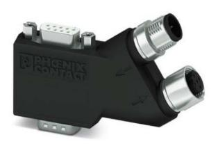
D-SUB bus connector SUBCON-PLUS-2902319 9 poles, D-SUB connector, 9-pin, male, with PG-D-SUB socket, assignment: 3, 5, 6, 8, two M12 cable entries (B-coded) below 35°. Bus system: PROFIBUS DP up to 12 MBit/s. Terminating resistor via separate M12 terminator.
