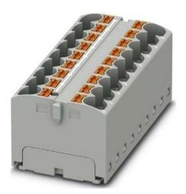
Distribution block 18p, 0.2-6qmm black/yellow - Feed-through terminal block 55,4mm 32A PTFIX 18X4...
