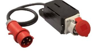
Inrush current limiter 400V 349.018, max. apparent power=11072 VA, mounting type=socket, rated uninterrupted current lu=16 A, short-circuit current limiter=yes, inrush current limiter 400V 3-phase Color: black Input: 1.5m H07RN-F 5G1.5 with CEE plug 400V/16A 5 -pin output: 1xCEE socket 400V / 16A, 5-pin voltage: U=400VAC, 50-60 Hz protection class IP44
