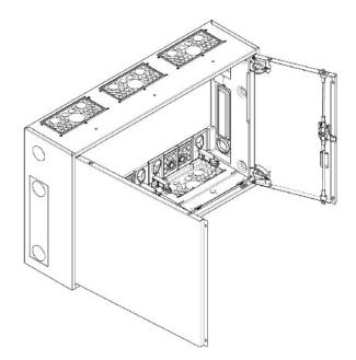
Wall housing IP54 version Luxembourg - Empty meter cabinet IP54 500x800mm S33L
