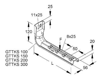
Hanging support and wall bracket 120x165mm 1.3kN - Wall- and profile console GTTKS 100 S
