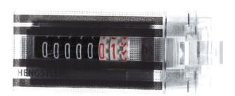
Hour counter 36V, Mounting Front assembly, Type analogous, Counting range 99999.99 h, Reset function without, Running indicator no, Number of characters 7, Input voltage 36 V, Voltage DC, Frequency of the input voltage 0 Hz, Width 52 mm, Height 52 mm, Degree of protection (IP) IP66
