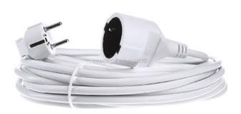
Power cord/extension cord 3x1,5mm² 10m, Connection 1 SCHUKO plug, right angle, Connection 2 SCHUKO coupling, Connector system system-bound no, Number of cores 3, Conductor nominal cross-section 1.5 mm², Length 10 m, jacket material Polyvinyl chloride (PVC), Temperature resistance 70 °C, Rated current 16 A, Rated voltage 230..250 V, Frequency 50..60 Hz, Coat color white, Spiral cable no, Protective conductor no, Degree of protection (IP) IP20, Oil-resistant to EN 60811-404 no, With cord switch no
