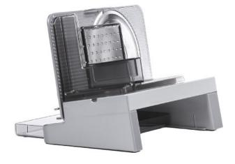
Multi-Cutter Compact Diagonal E 16 si Housing material metal, blade diameter 170mm, cutting thickness adjustment up to 20mm, inclined support table, basic color silver, metal design, inclined, serrated blade, safety momentary and permanent switch, removable carriage, 65 W eco motor, carriage travel approx. 18 cm, cuttings collection tray, cable depot, weight: 3.0 kg, colour: metallic silver
