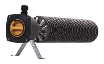
Finned tube heater 230V, 1000W, 700mm RRH TR 1000 power 1000W, fin diameter 120mm, voltage 230V, automatic temperature controller, protection class (IP) IP67, height 184mm, width 145mm, length 700mm, finned tube heater with temperature controller, finned tube and mounting feet made of stainless steel material no 1.4512, connection box made of glass fiber reinforced polyamide.
