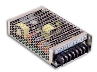
DC-power supply 85...264V/24V 156W Voltage type of supply voltage AC, 1st secondary output voltage 24 ... 24V, Max. output current 1 6,5A, Short-circuit-proof, Rated supply voltage at AC 50 Hz 85 ... 264V, Rated supply voltage at AC 60 Hz 85 ... 264V, Power output 156W, Type of electric connection Screw connection, Direct mounting possible, Width 97mm, Height 38mm, Depth 152,5mm, Degree of protection (IP) IP00
