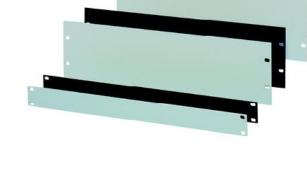
19" blanking plate 30118307 width 483mm, height 354.8mm, number of height units (HU) 8, material aluminium, surface design other, anodised aluminium, color light gray (RAL 7035), 19- Please order fastening material separately
