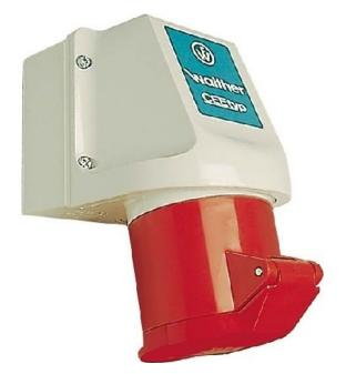
Wall socket 32A, 5-pin, 400V, IP44 - Wall-mounted CEEsocket CEE-Socket 32A 131
