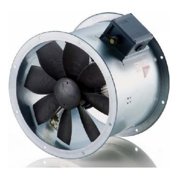
Axial tube fan ex-protected DN 300 - Ex-proof ventilator 3410m³/h 240W DZR 30/2 B E Ex e
