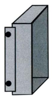
Extension for chute 531 by 60mm - For ventilator 88-532-KG
