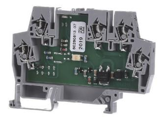
Optocoupler terminal 24/3-30VDC 3A 859-730 input voltage 15... 27V, type of input voltage DC, output voltage 3... 30V, type of output voltage DC, rated operational current le 3A, type of digital output electronic, with LED display, Optocoupler module Rated input voltage DC 24 V Output voltage range DC 3 - 30 V Limiting continuous current 3 A 2-wire connection 6 mm width grey
