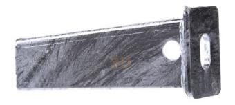
Bracket for cable support system 110mm Length 110mm, Width 40mm, Height 45mm, Suitable for cable management system width 50 ... 100mm, Model Wall- and profile console, Angle 90 ... 90°, Load bearing capacity 2,5kN, Suitable for circuit integrity, Material Steel, Material quality Other, Surface protection Hot-dip galvanized, Colour None
