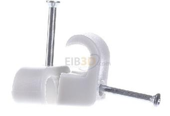
BI claw clamp size 2723/25 round shape (for round cable), suitable for diameter 7 ... 11mm, width of opening 6.6mm, height of opening 5mm, material plastic, surface untreated, color gray, with nail, nail length 25mm, Nail diameter 2mm, hardened steel nail, BI claw clip made of impact-resistant polyethylene, halogen-free
