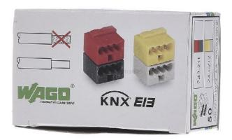
Bus coupler terminal dark gray red screwed. 243-211 Number of clamping points 8, Cable diameter 0.6 ... 0.8mm, With actuating levers, Other color, Rated voltage 100V, Rated current 6A, Suitable for solid conductors, AWG range 22 ... 20, 4-wire socket terminal for Individual soldering pins for KNX Ø 0.8 mm pitch 5.75 mm 2-pin
