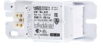
Ballast 18W TC-D/-T 163763 Conventional version, for lamp type TC-D, for lamp type TC-T, suitable for number of lamps 1 ... 1, suitable for lamp power 18 ... 18W, nominal voltage 230 ... 230V, protection class I, length 85mm, width 41mm, height 28mm, vacuum-impregnated in polyester resin, plug-in terminals 0.5-1 mm², for automatic lighting wiring: insulation displacement terminals for cables H05V-U 0.5, tw 130
